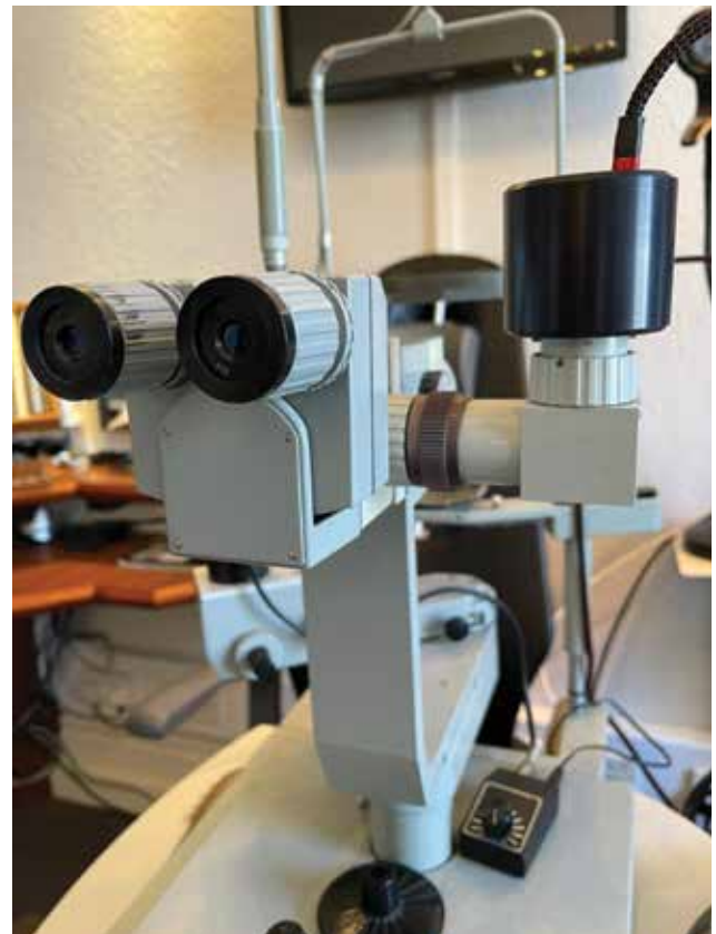
Brian's Zeiss Slit Lamp with Custom Digital Camera and custom-made LED Lamp
